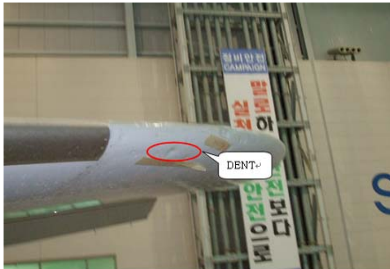
[Photo 4] Damage to horizontal stabilizer 1
