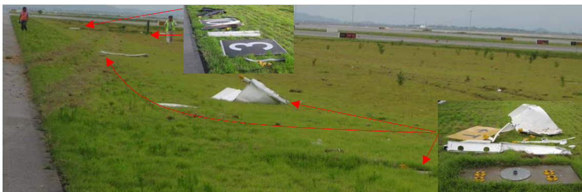
[Photo 8] Runway distance marker sign damaged
