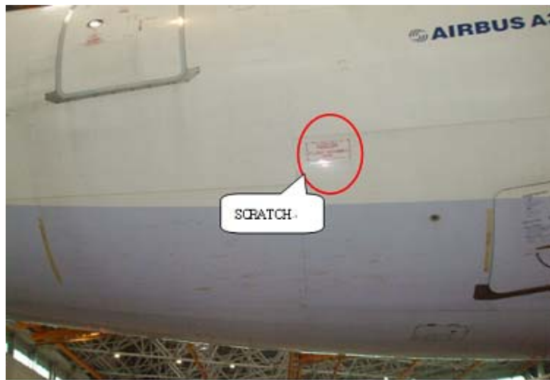
[Photo 3-1] Damage to lower right surface of fuselage in the rear
