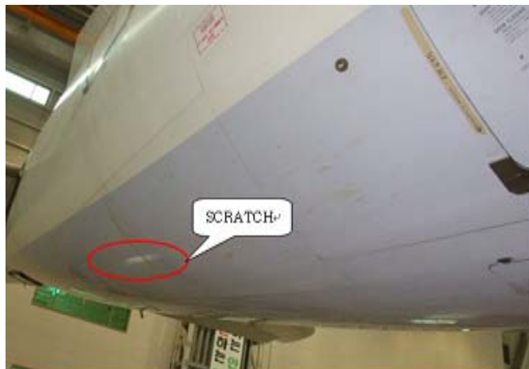
[Photo 3-2] Damage to lower right surface of aft fuselage
