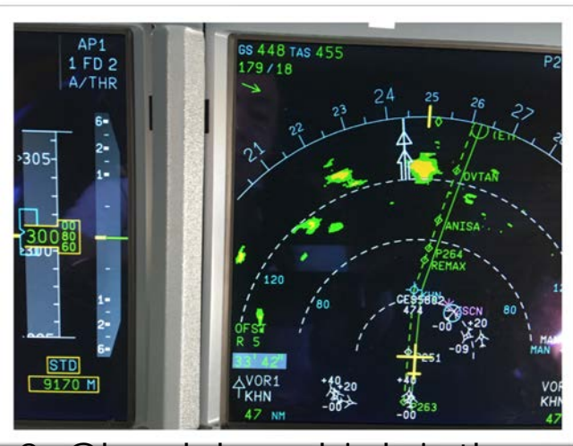
2. Check how high is the wet top, my alt and above (Manual)
